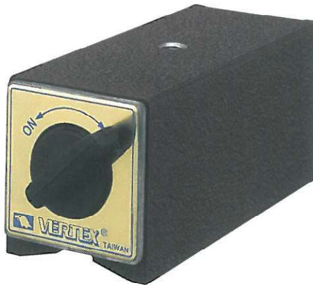
ORDER NO. VMB-11 MAGNETIC BASE ONLY M8X1.25p,140kgs
