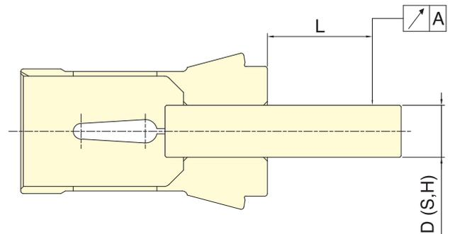
Note: Collets chuck are conformed to DIN 6343 Class2.
