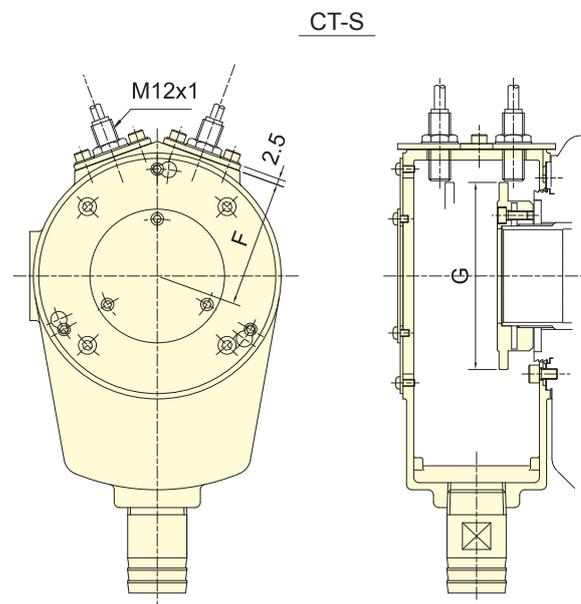
Coolant Collector with Detecting Ring
