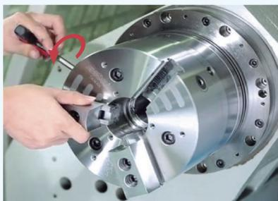
2. Turn T-handle clockwise to tighten and the jaw is locked.
